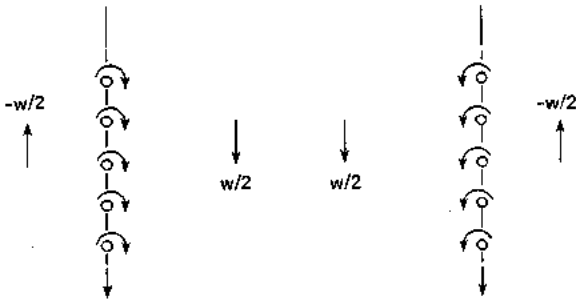
Figure 11.-Velocities relative to vortices after development (steady flow).
